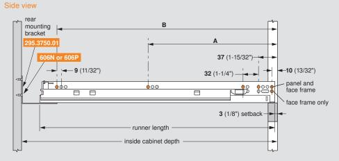
NOTE: The orange dots indicate fixing screw locations required to meet specified load ratings.
